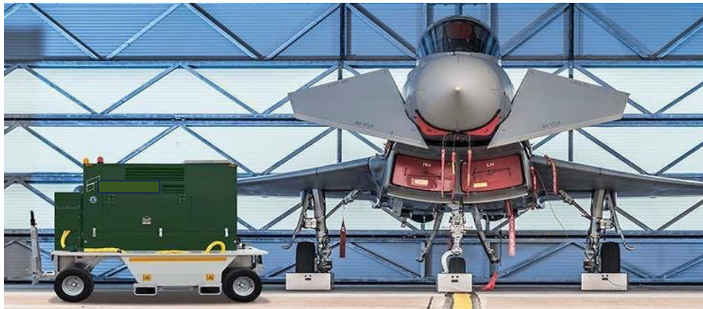
Air Starter Units- Canada
